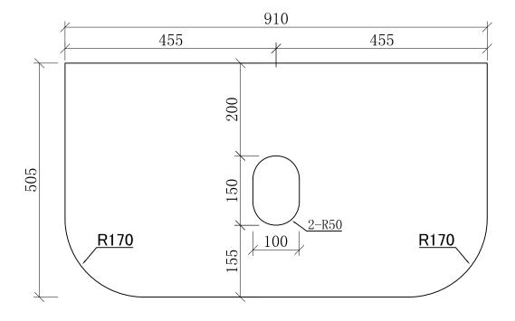
Material: Silica Free Scratch And Heat Resistant Glass Stone Precut basin hole included Front and side of stone is polished
