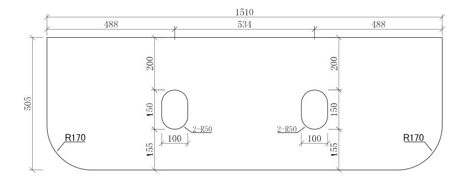
Material: Silica Free Scratch And Heat Resistant Glass Stone Precut basin hole included Front and side of stone is polisheD
