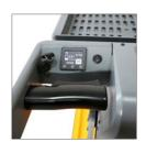
New design steering handle which keeps operation easier and flexible Multi-function display, shows battery status, fault code and technical data Turtle speed button, convenient for narrow spaces
